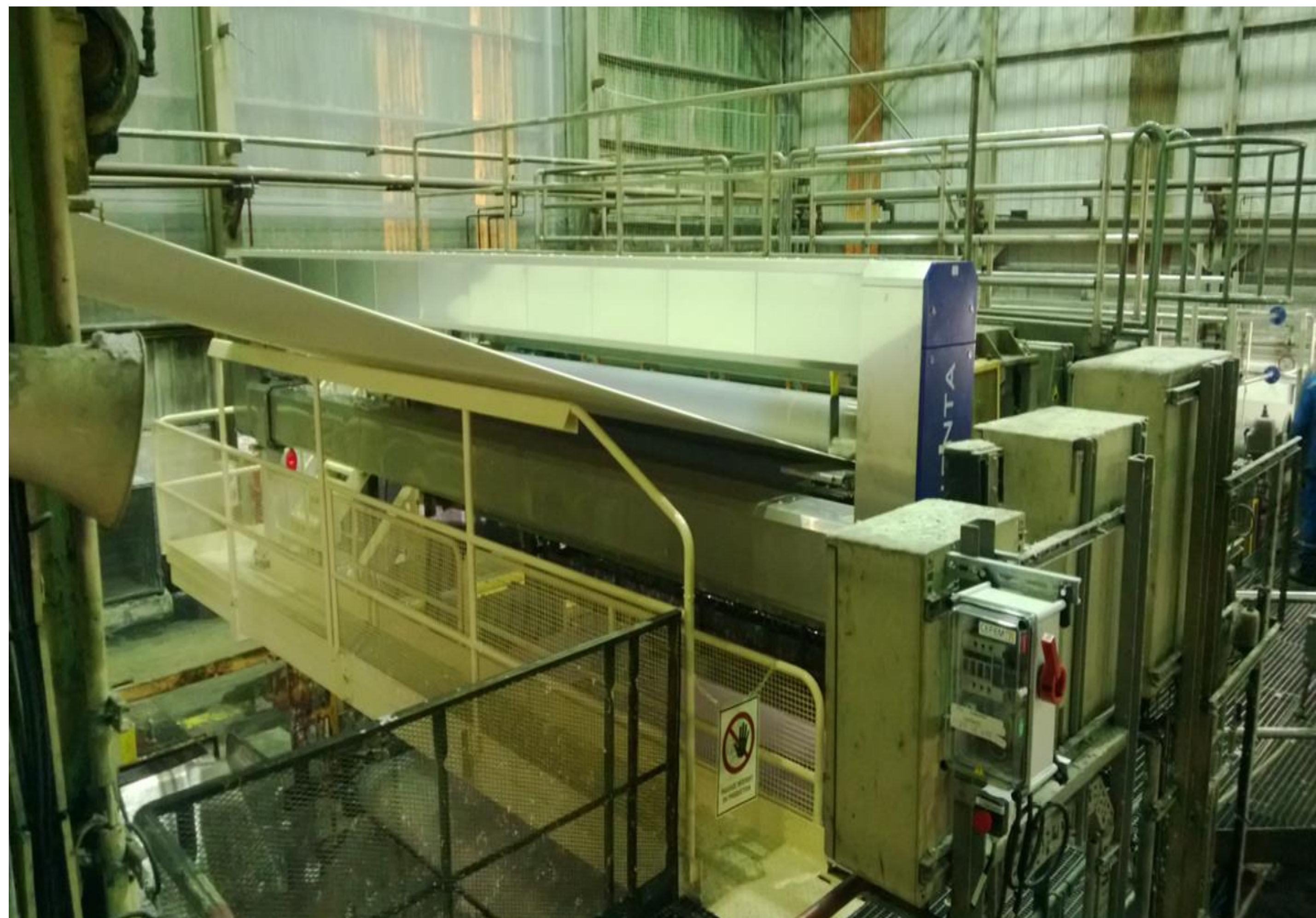
Pulp mill installation, dry end scanner
