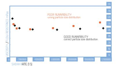
LESS WEB BREAKS AT HIGH OPERATING SPEEDS AND LOW BLADE PRESSURES. NOTE! NO DIFFERENCE AT LOW SHEAR RATES.
