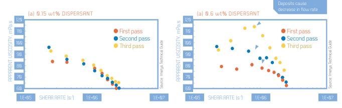
ACAU SLIT SHOWS EFFECT OF DISPERSANT DOSE ON SHEAR STABILITY OF COATING COLORS. KAOLIN + DISPERSANT, 10 PPH LATEX, 0.3 PPH CMC, 59 WT SOLIDS
